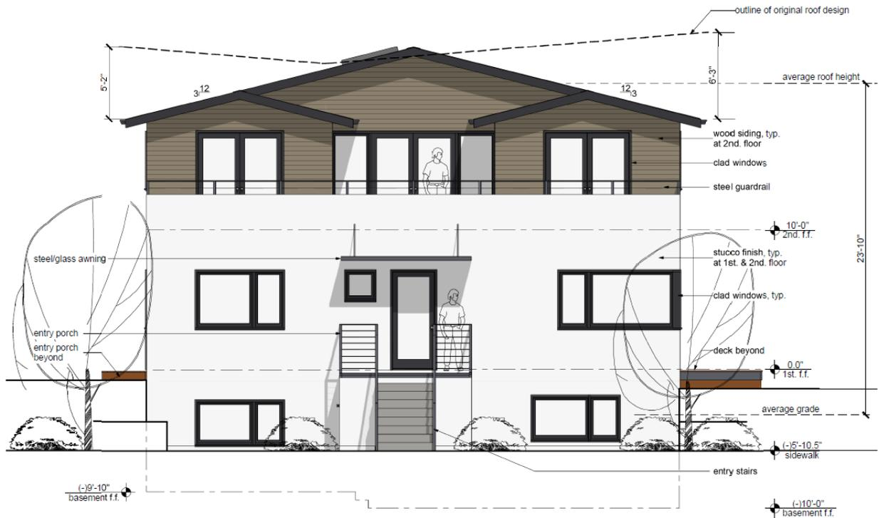
① Proposed West Elevation - Front
