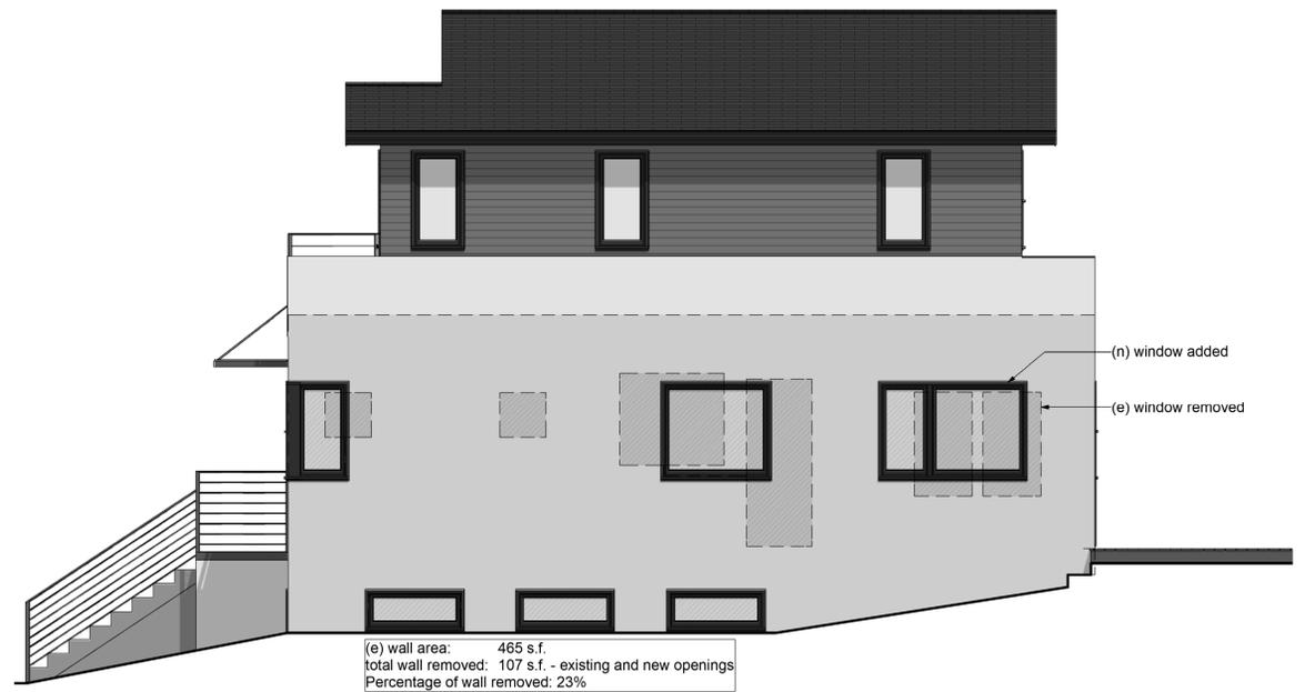
4 Proposed South Elevation - Right Side
